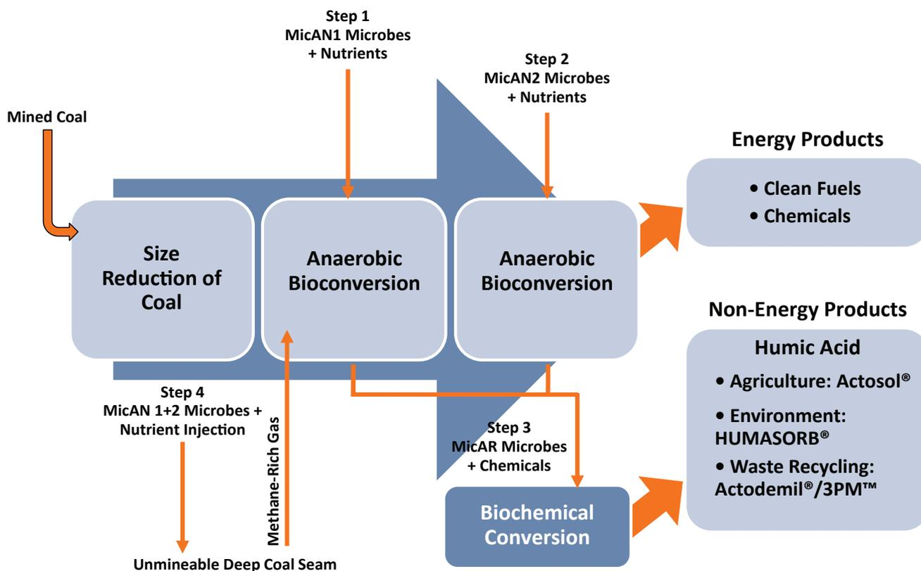
**FIGURE 1. Integrated MicGAS™ biotechnology process flow scheme**
